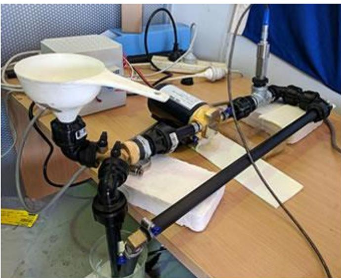
The test rig is designed such that we can replicate scenarios likely to cause significant risk of failure in a time spectrum of minutes to hours
